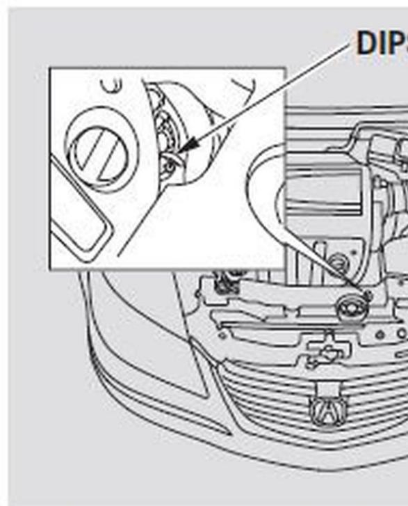
2. Remove the dipstick ( ) from the transmission with a clean cloth.
