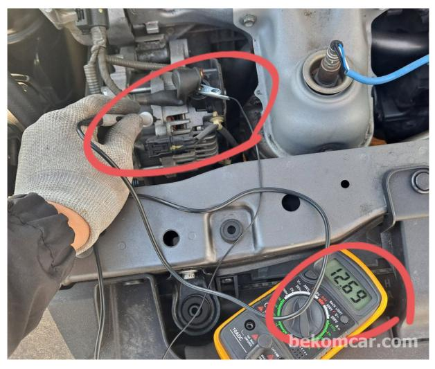
As shown in the above photo, the voltage generated from the alternator while the engine is running is just 12.69V. This is the clear message that the alternator is dead. But the dealer said the car is is perfect condition. Always trust but verfiy in any used car purchase inspection.
