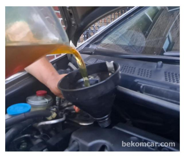
Put new engine oil using the funnel-
