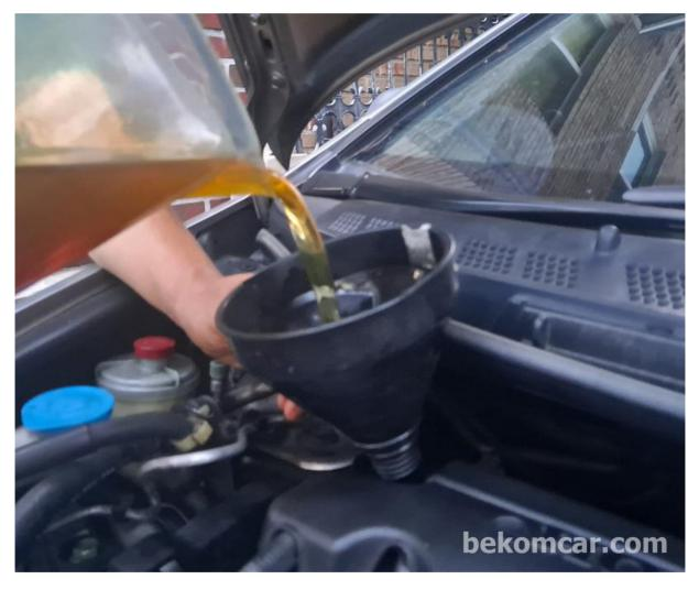
Honda manual requires you to replace the engine oil filter and air filter in every 20,000 km. Use your common sense, inspect the air filter and replace them appropriately. Also, try to use genuine Honda engine oil filter. This process is for engine oil only and does not replace engine oil filter or the air filter.
