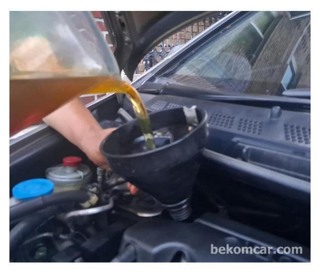
Put new engine oil using the funnel-
