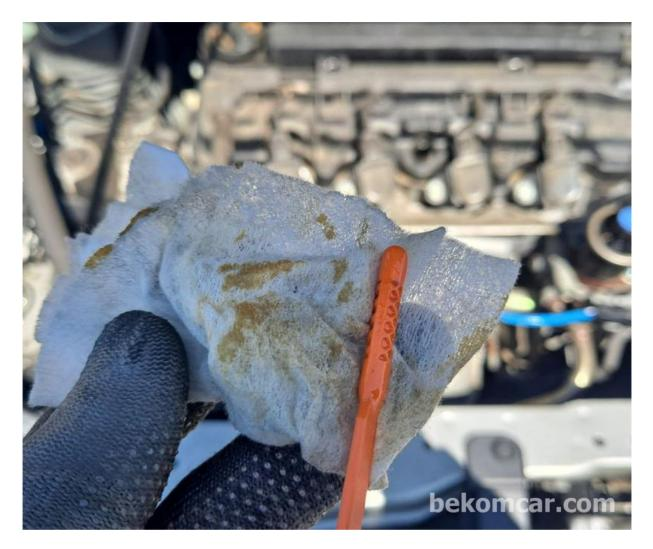
Double check the engine oil level-
